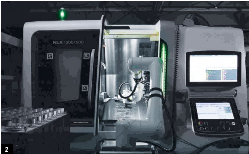
1. NLX 1500 turning center and MATRIS Light from DMG MORI are used to machine the components of the SATELLITE FIRE BASE. 2. The MATRIS Light looks after automatic workpiece handling overnight. This makes unmanned night shifts and more productive machining possible.
