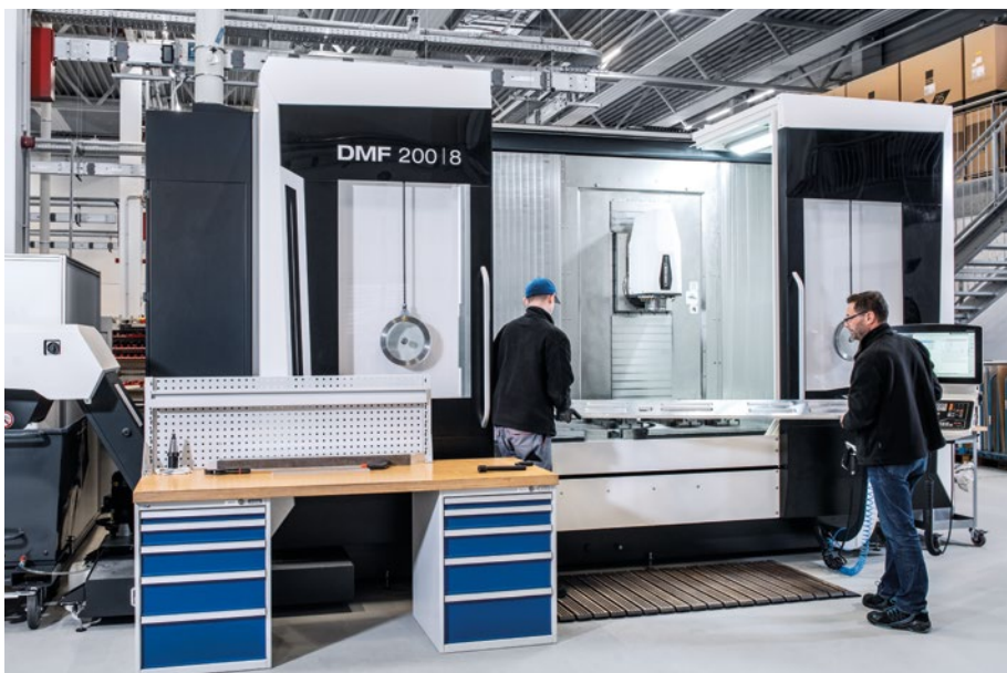
The DMF 200 | 8 is used to manufacture long, high-precision profile components.
