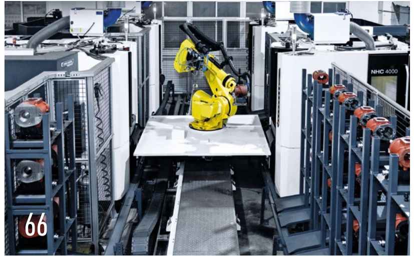
Xiamen: the production of housings for air compressors takes place on two production lines, each consisting of four NHC 4000s and a mobile robot.
