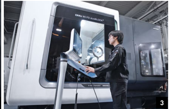
3. The DMU 80 FD duoBLOCK 5-axis Turn & Mill machine can replace several turning centers, milling centers and gear cutting machines.
