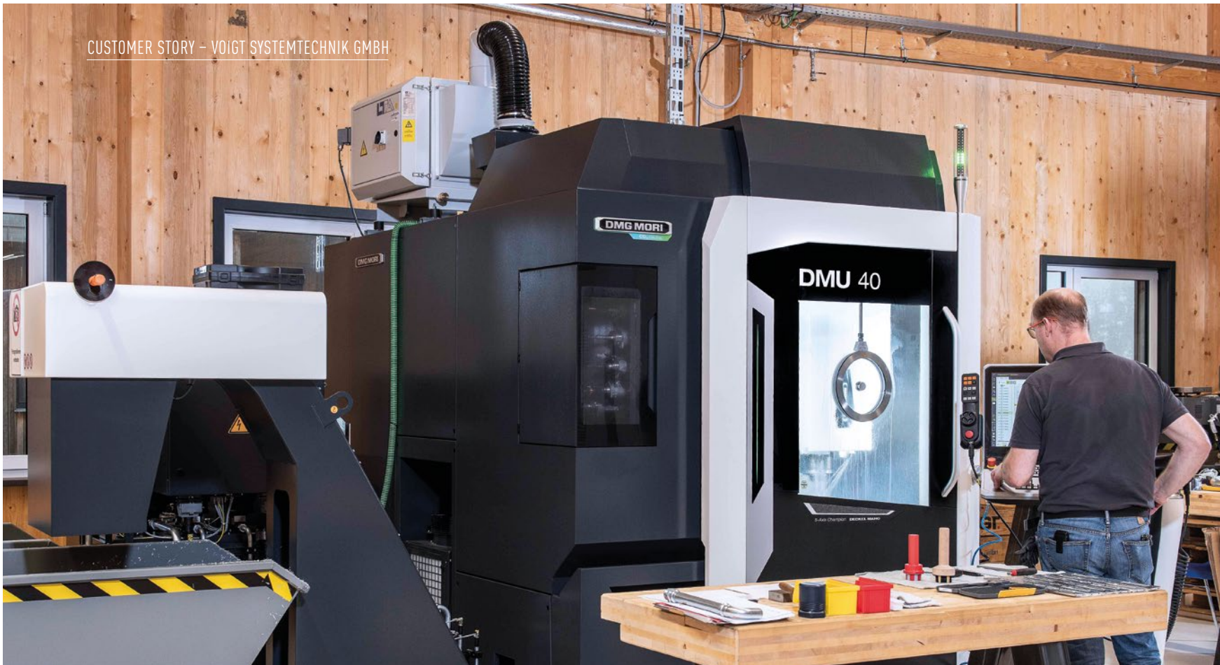
The DMU 40 is a true space saving wonder. With a footprint of less than 5.1m 2 and a width of less than 2m, it offers space for workpieces up to ø500 × 445 mm and 300kg. The DMU 40 PRO is fitted with an automatic side door at Voigt Systemtechnik to prepare it for autonomous operation at a later date.
