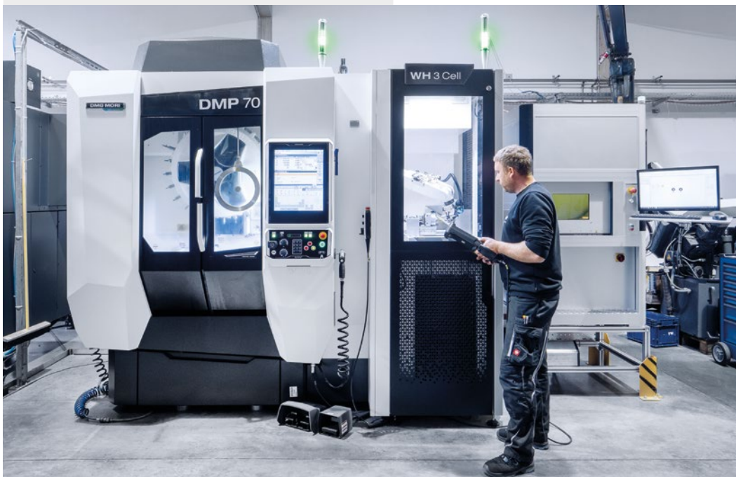
Minimum space requirements: DMP 70 and WH 3 Cell occupy less than a 9 m 2 footprint. Depending on the workpiece dimensions the WH 3 Cell offers space for over 1,000 workpieces.
