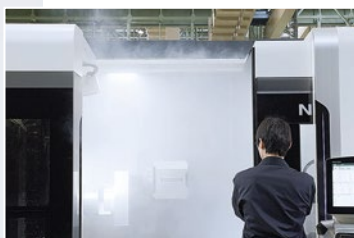
Inside comparison: Without mist collector
