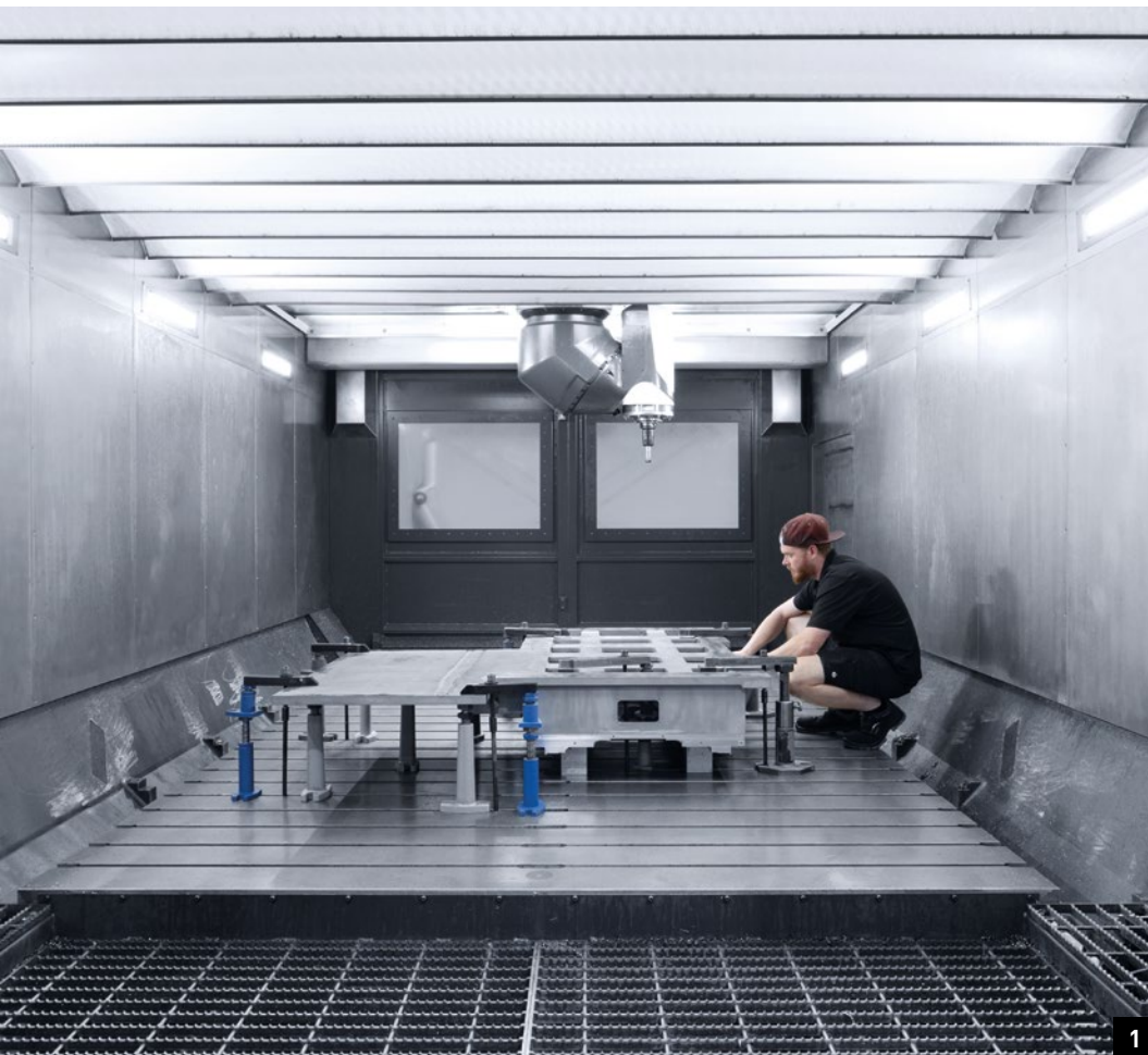
1. Amongst other things, Schittl manufactures high-precision machine beds on the DMU 340 Gantry 2.+3. Schittl has been able to achieve automated 5-axis machining on a CMX 70 U with PH 150. The PH 150 has over 8 positions places for unmanned or minimally manned manufacturing.
