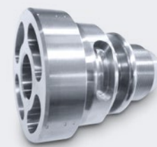
CONNECTOR Industry: Automotive Material: Steel C45 Dimensions: \varnothing 80 \times 95 mm Machining time: 9 min
