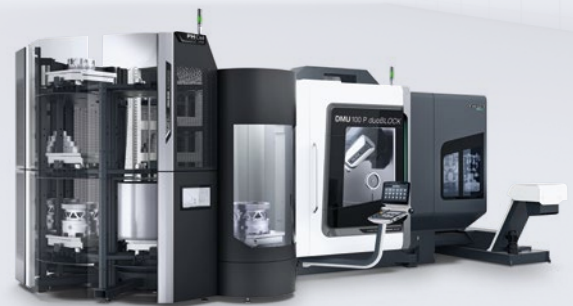
PH Cell 2000 (Up to 21 pallets and 2,000 kg handling weight)
