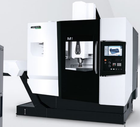
M1: 550 mm X-axis travel in a 5.9 m 2 footprint (w/o chip conveyor)
