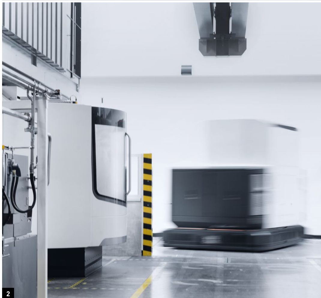
1. The PH-AGV 5000 transports components weighing up to 4,000 kg from a decentralized storage unit to the machine and loads them directly onto the pallet changer. 2. A laser that scans the area in the direction of travel ensures the safe operation of the PH-AGV 5000, which can travel at speeds of up to 9 km/h.
